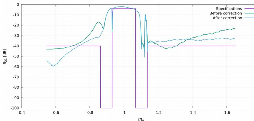
Figure 2: Experimental  $S_{21}$  of wide band filter in L-band on LiNbO<sub>3</sub> substrate. The frequencies have been normalized due to confidentiality. In purple, the response without the bonding between the grounds. In green, the corrected response by the wire bonding.
