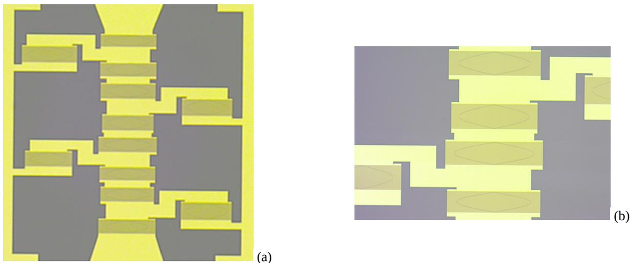
Figure 1: Final design of the ladder filter. (a) Observation of the 4 T cells in the design and (b) Enlargement of some resonators to see the apodization of each of them.
